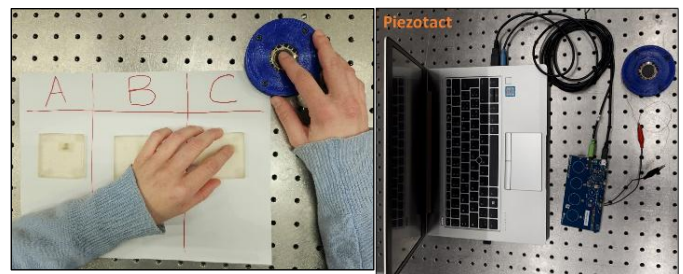
Fig.1 Discrimination test on rendered textures by the Piezotact tactile device
