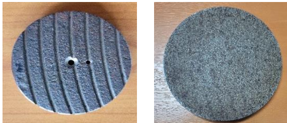
Fig.1 (Left) surface with grooves and shot-blasting (Right) surface solely subjected to shot-blasting
