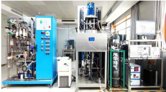
Fig. 1 A tribometer was used to simulate the deep-sea environment and was equipped with a seawater cycle loop and an electrochemical workstation.
